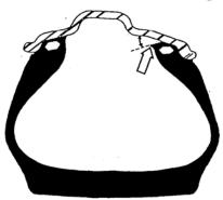
Extreme stress may be placed on beads forced into the rim flange in a distorted manner, which may cause fatigue in tire components and result in tire failure.
